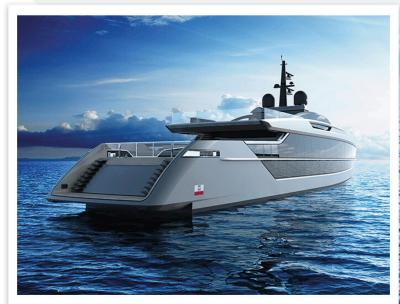
The three MTU 16V 2000 M94L water jets give her a top speed of 28 knots and a cruising speed of 24. At cruising speed the Tankoa \$533 Saetta's range is 600 miles; this doubles to 1,200 miles at a cruising speed of 17 knots.
